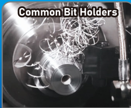
Chips get wrapped around the workpiece.
