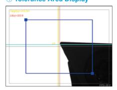
The tolerance area is displayed on the screen for easy adjustment of the boring bar diameter.
