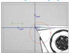
Wear and chipping on cutting edge can be inspected.
