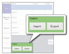
Tool data is imported and exported in the CSV file format. Use to move data to other equipment, or to synchronize tool data between multiple presetters.
