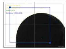
The cutting tool's profile is plotted by rotating the spindle 360 degrees.
