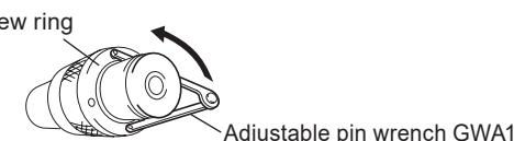
3. When adjustment is completed, tighten the two screws in the screw ring with a hex wrench.
