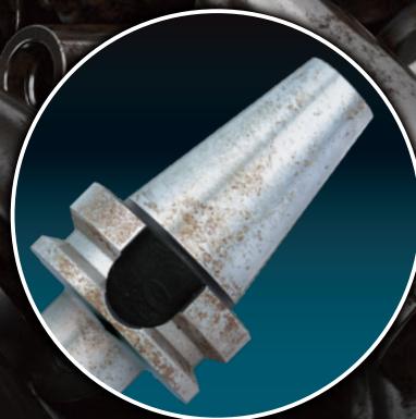
Rusted surface of standard product
