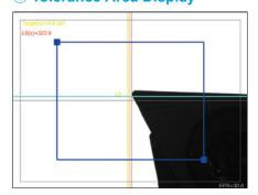
The tolerance area is displayed on the screen for easy adjustment of the boring bar diameter.
