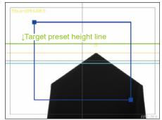
In "Adjustable Mode," the target preset height is displayed on the screen with a green line. Use to offset for cap compression when using collet holders, etc.
